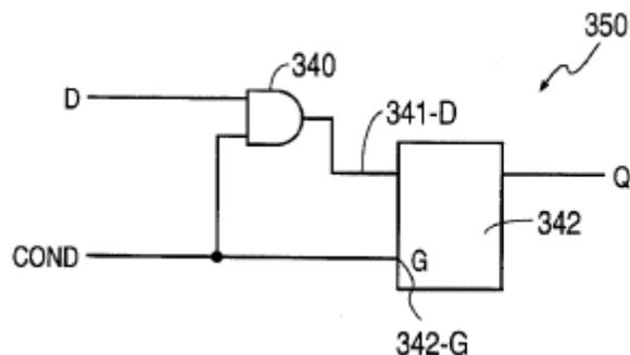
*Id.* at Fig. 8A. In this hardware component description, the rectangle marked with 342 represents the level sensitive latch, itself. Consistent with the above description, the latch's input (341-D) is the logic AND (340) of input D and condition COND; and, its gate (342-G) is condition COND. *Id.* at 22:12–23.
